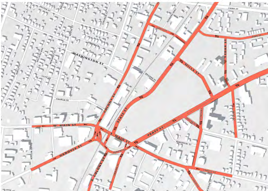
Existing street network (1-way traffic): The current City Center circulation network with a series of one-way streets that confuse drivers.
