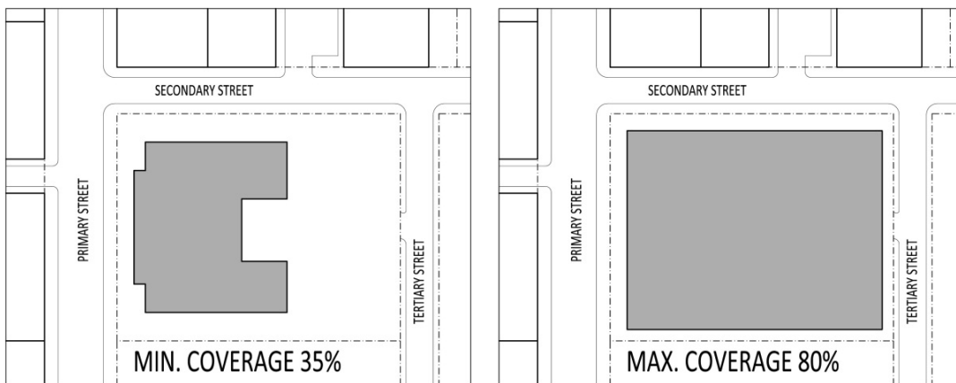
Figure 213-42. Minimum and Maximum Lot Coverage for all permitted uses other than Multiple-Family Dwellings
