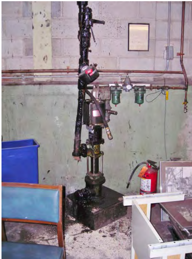
Photograph 17 – Ink pump coated in ink in southeastern portion of former paper storage room. Speedy-Dry appears to be spread on the floor adjacent to the pump.
